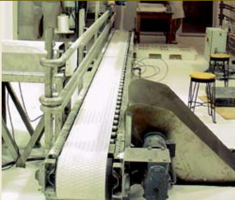
Unique formed rigid design of all galvanized steel, this belt conveyor offers the advantage of a greater span potential, combined with a low profile height of 12 inches where space is limited. Featuring flexibility by design, conveyors are available with various belt widths and include spool idlers. Quick-change key slots, spaced on one-foot increments, allow for many combinations of idler spacing.
