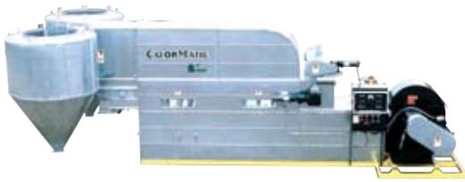
The CalorMatic® is modern technology that makes heat processing of a variety of free-flowing materials simple, practical, and profitable. Natural gas, propane, diesel fuel, or alternative fuels, in an efficient burner, heats air which passes through the fully perforated bed of the product chamber. The product is gently, thoroughly, and evenly heated to a consistent finish.
