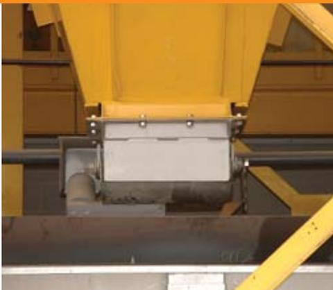
Complete line of Simplex and Duplex bin gates constructed of heavy gauge steel plate, abrasion-resistant or stainless steel. Any model can be adapted for pneumatic operation. Easily attached to hoppers, bins, and chutes.
