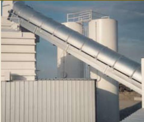
Heavy-duty formed channel galvanized steel frame features tubular cross braces and unique diaphragm squaring plate. It will support 565 pounds per linear foot when supports are spaced on 20-foot centers. Belt widths from 14" to 72", conveyors are of all bolted construction with channel splice connection for easy installation. Capacities 300 – 88,000 BPH (8 – 2250 MTPH).
