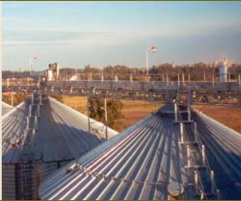
Designed and engineered to provide long life and durability with minimum maintenance. Fully enclosed, dust-tite, and quiet operation assures fast, gentle movement of bulk materials. Extra heavy chain features UHMW polyethylene faced flights for positive flow and reduced friction. Available in horizontal and incline models. Capacities 2000 – 35,000 BPH (50 – 948 MTPH).
