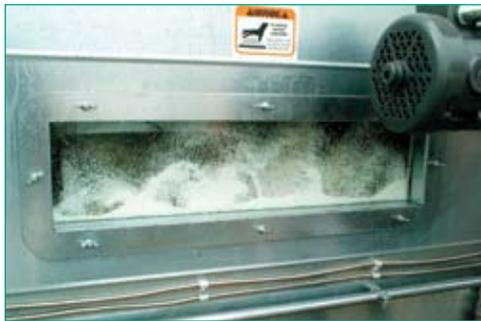
Product is gently floated and turned in a fluid bath of hot air without contact to flame, while positively and continuously moving with our internal conveyor system.
